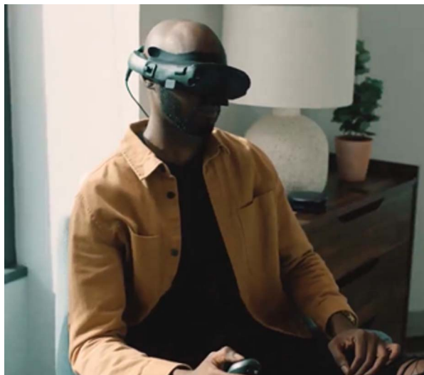
FIGURE 1. A patient wearing the HMD with the light shield mounted to prevent light leakage. Figure 1 can be viewed in color online at www.glaucomajournal.com .
