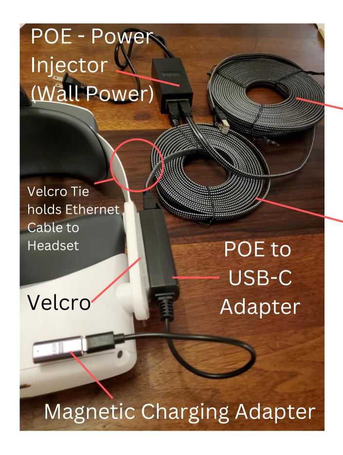
Ethernet Cable #1 (Goes to the Ethernet port in the Wall).
