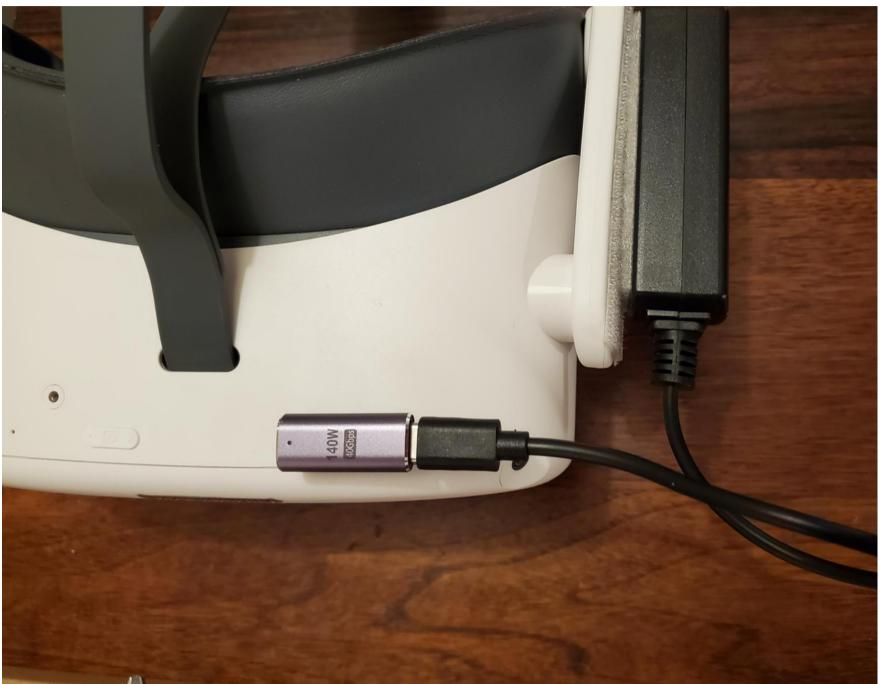
USB-C Side of the connector (Goes into the USB-C Power Slot)
