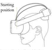
Start with the headrest in the up position and move it downward over the back of the head.
