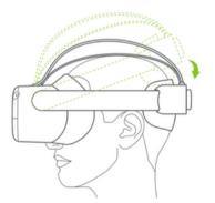
Rotate the strap down over head and turn the headrest knob clockwise to secure fit.
